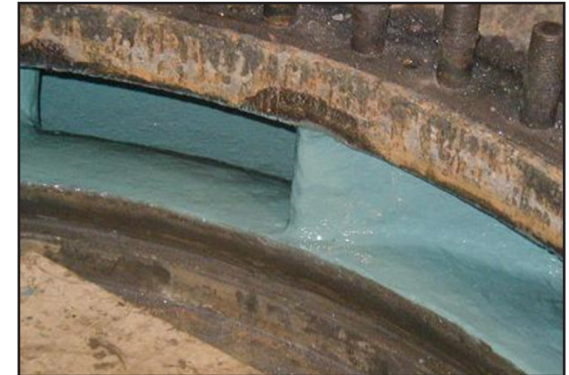
Top coated with 2 coats ARC S2
